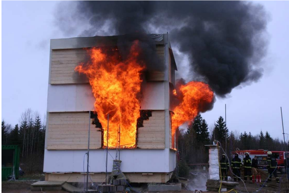
Figure 2.15 Fire has spread to the facades
