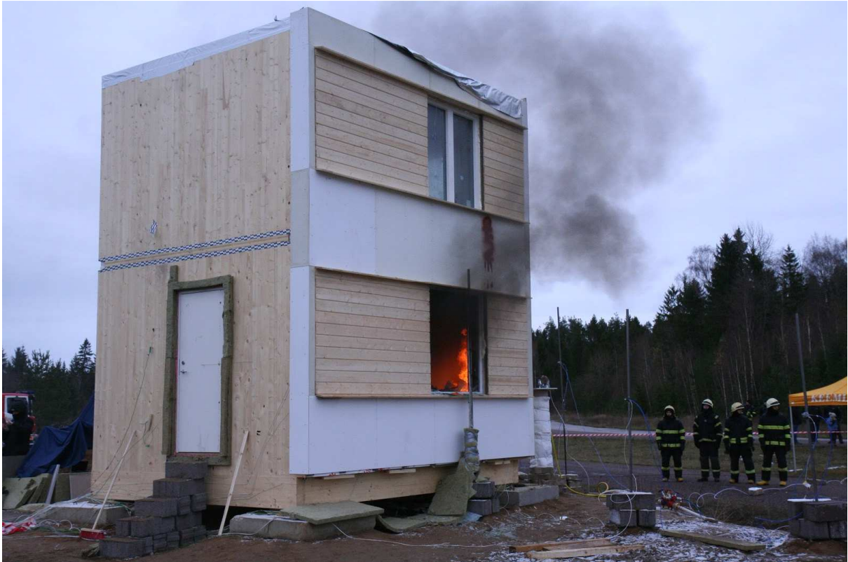
Figure 2.13 After breaking the first window the fire starts to develop
