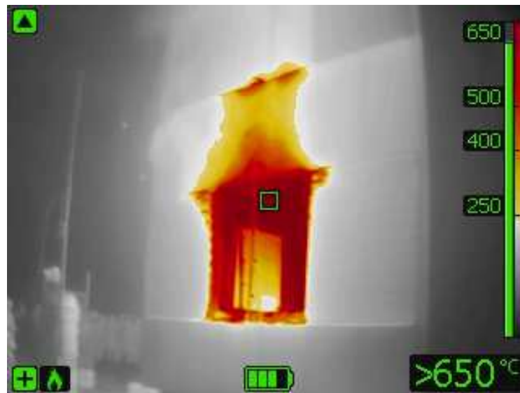
Figure 3.9 Thermal image showing wall temperature inside the compartment
