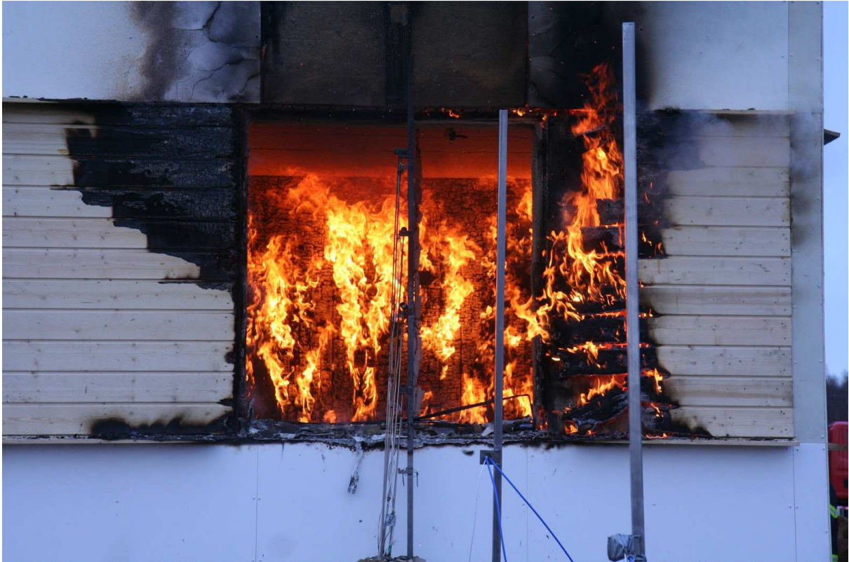
Figure 2.18 The second layer of CLT is burning
