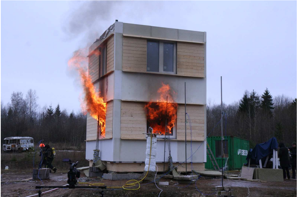
Figure 2.14 Flames are reaching the facade of the upper floor
