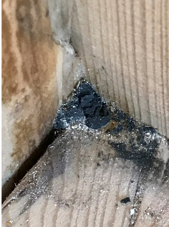
Figure 3.21 Intumescent paper Tenmat FF104E after reacting to heat
