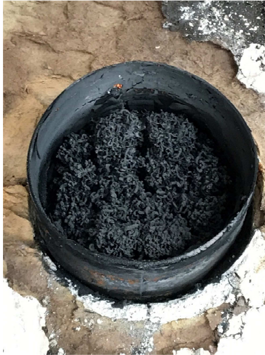
Figure 3.26 The intumescent material used in the damper in its expanded form
